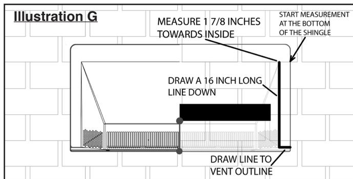
flange, measure towards inside 1 7/8 inches. Mark roof. From that mark, draw a straight line 16 inches down. Make another line to the vent outline. Repeat on other side.
