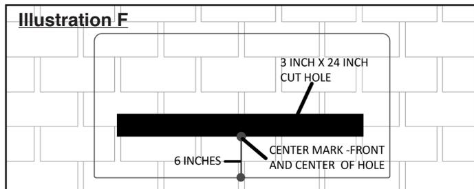
The hole should penetrate the shingle, underlayment, and the decking. Do not cut the rafters.
