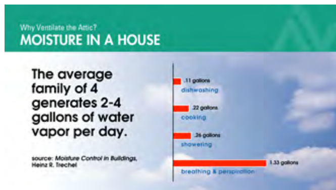
Moisture generated by occupants of the house; photo courtesy of Air Vent Inc.
