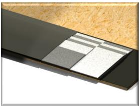
The second set of shingles should mirror that of the first set, except only four layers thick to create a stepping down towards the roof deck. Continue with the shingle overlapping as specified by the shingle manufacturer, though the second set will not protrude from the roof deck as far as the first set will.
