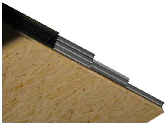
This is what the finished product will look like when the transition is complete. Now the climate-appropriate shingle underlayment (whether it is felt or a waterproofing membrane) matching that used underneath the vent and over the vent, and subsequent starter course shingles and first courses can be installed.
