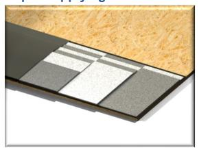
The third set of transition shingles will mirror that of the first and second sets, but only be two layers thick.
