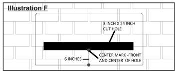
The hole should penetrate the shingle, underlayment, and the decking. Do not cut the rafters.
