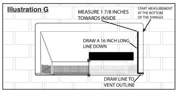
flange, measure towards inside 1 7/8 inches. Mark roof. From that mark, draw a straight line 16 inches down. Make another line to the vent outline. Repeat on other side.
