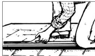
6. Strip away cut-out scrap from slot.
