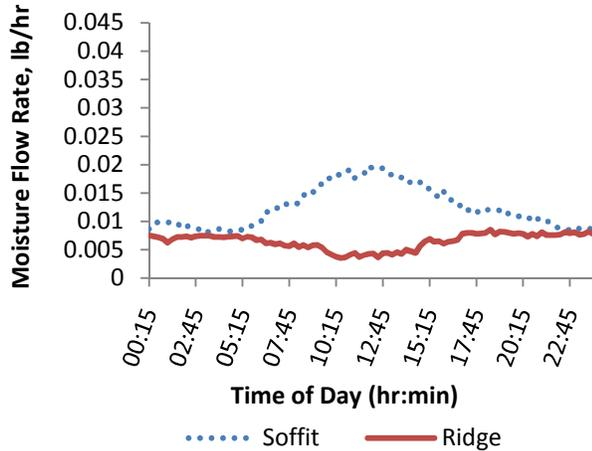
Figure 11. January moisture flux for the attic environment
