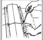
8. Align joined CRV Ridge Vent over slot, fasten in place.
