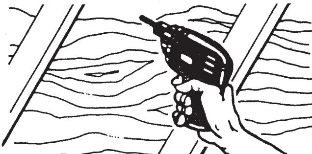
**3. CUTTING THE HOLE:** Draw a circle 14.5" in diameter using the guidehole as the center. A template is provided on the back of the carton for drawing the circle.
